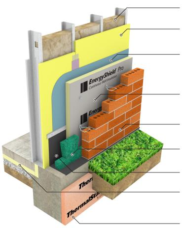
Fiberglass batt cavity insulation
